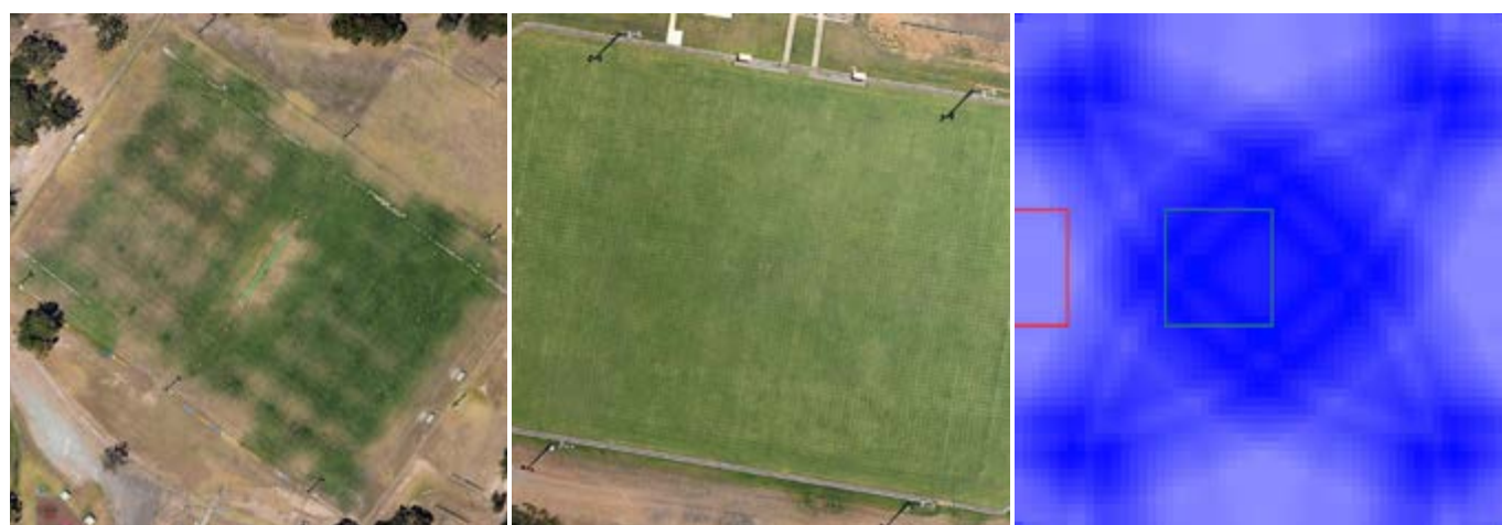
Figure 28. Both these irrigation systems apply water unevenly. While uneven watering is obvious on some sites (left), it is not always visually obvious (middle). However, a densogram (right) from a detailed irrigation assessment clearly identifies the problem. Improving the systems on these fields would achieve better turf and more than 20% water savings.
