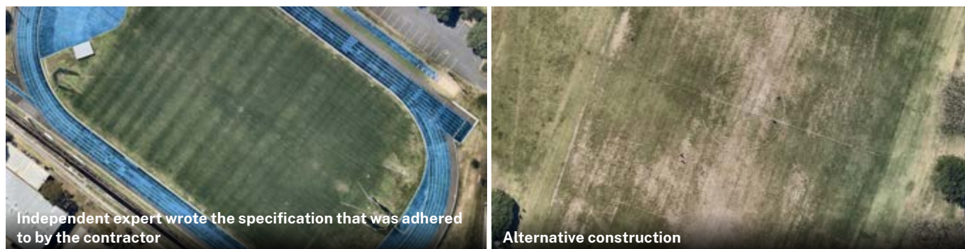
Figure 20. Both these fields were reconstructed in 2021-22. After 2 winter seasons of use, the performance contrast is stark for playing surface quality, carrying capacity, and visual aesthetic. The field on the left was rebuilt according to best practice by a contractor complying with a specification written by an independent designer.
