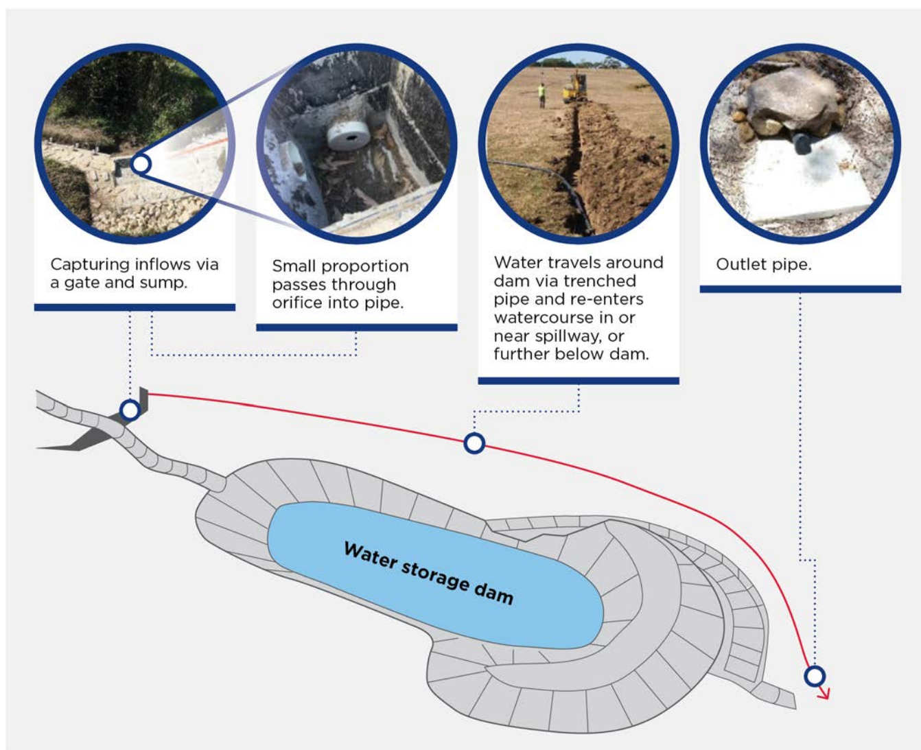
Figure 13. Low-flow bypass technology 13
