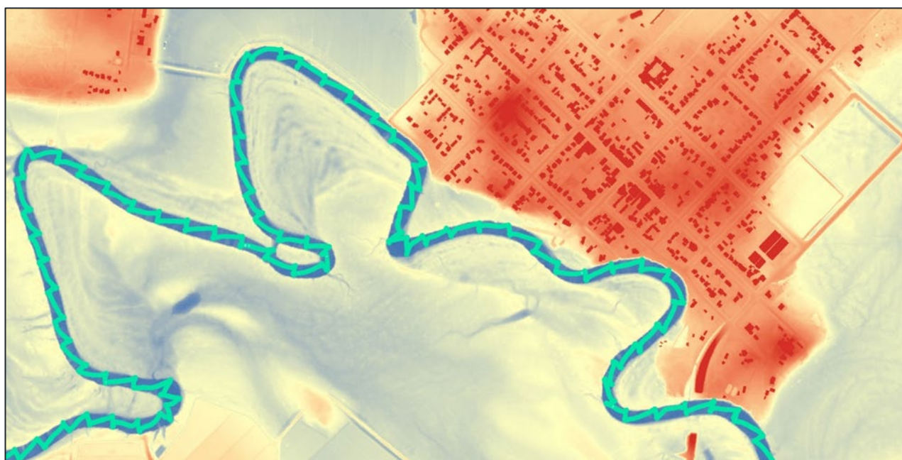
Figure 4 - Example of Z shaped survey pattern and 100 m cross section interval for a section of the Murrumbidgee River near Balranald (overlain on LiDAR floodplain topography data).
