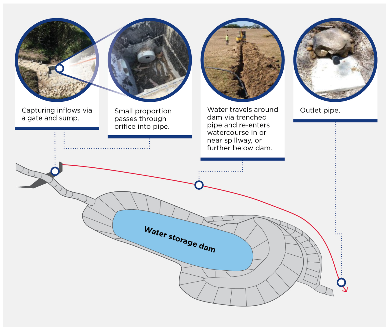
Figure 12. Low flow bypass technology 17
