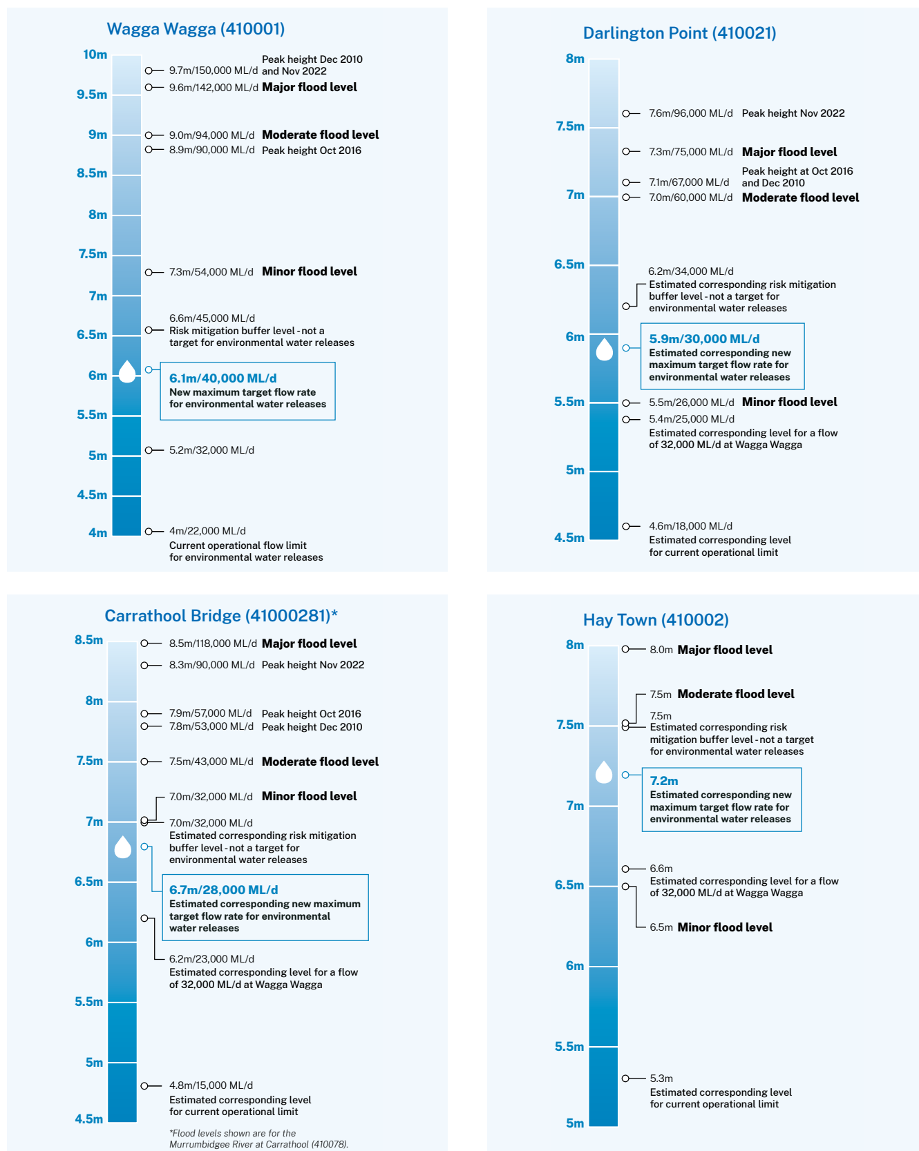
Figure 5 – Gauge board diagrams showing flow limits and flood levels
