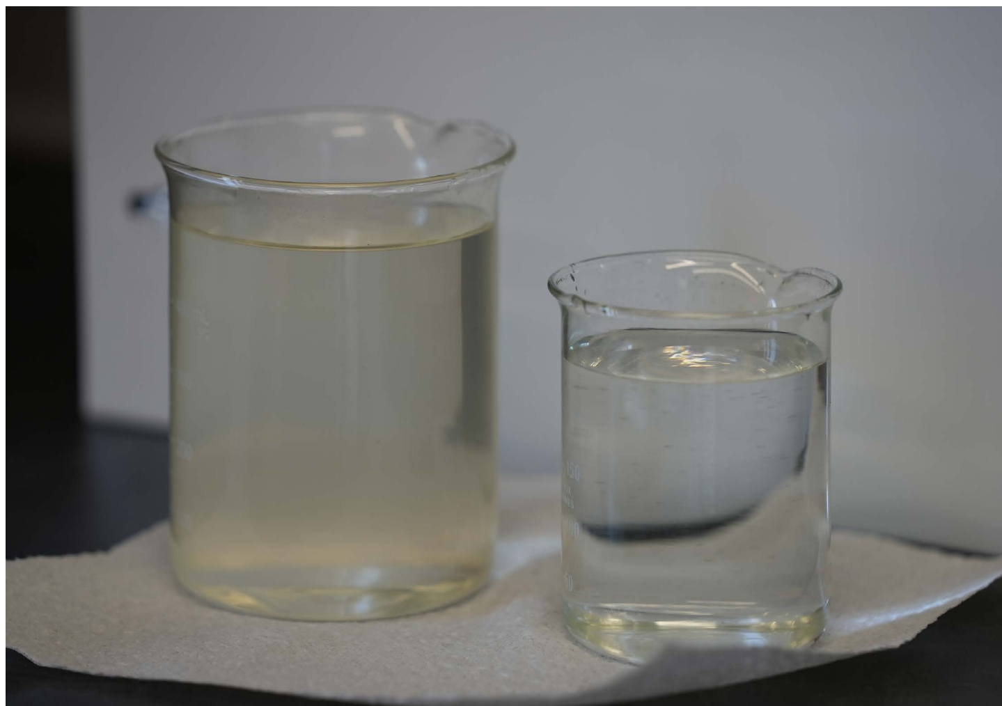
Image: Plants treat water to remove turbidity, as shown in the jar on the left, so it is clearer and cleaner like the jar on the right. Photo: Vince Bucello
