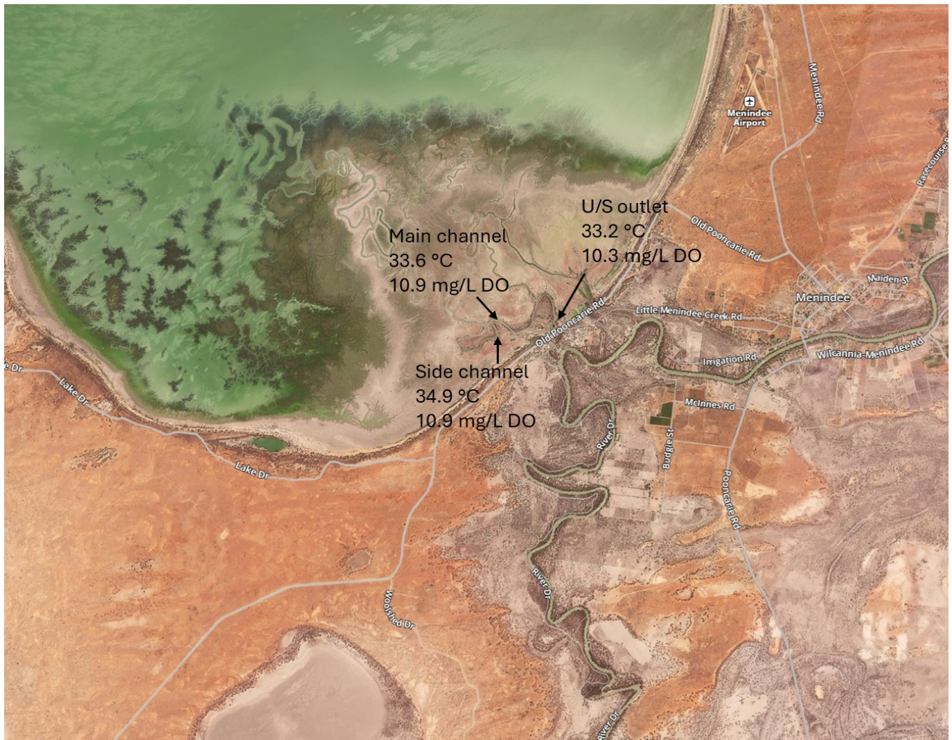
Figure 2 – Temperature and dissolved oxygen (DO) results taken from handheld readings on 28 January
