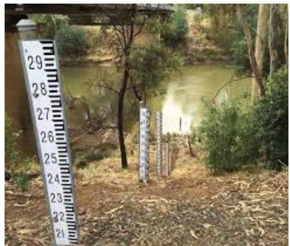
Figure 2. Sectional boards installed on a slope
