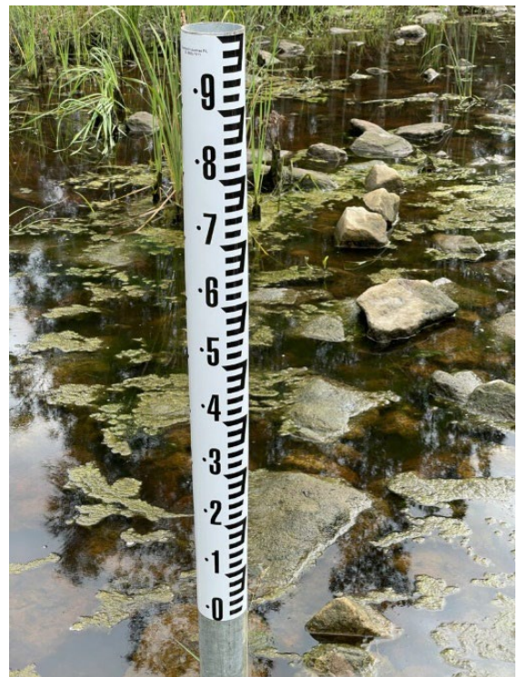
Figure 3. Half round gauge plate attached to 80 mm galvanised pipe
